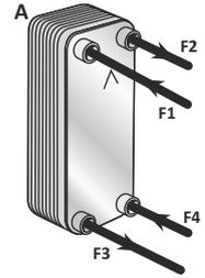
BPHEs with UL approval for use with CO<sub>2</sub>, according to UL files section II or VI. When used with CO<sub>2</sub>, the system should include a pressure relief valve on each side of the BPHE. The pressure relief valve must open if the system pressure reaches 0.9 × design pressure.
