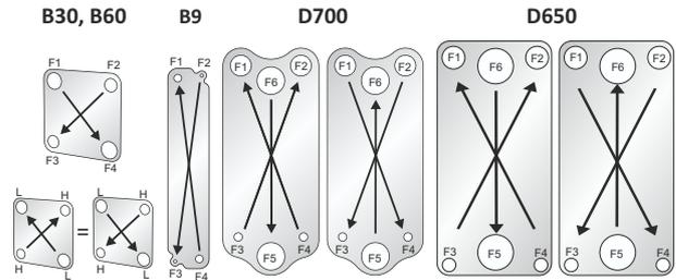
The B9, B30, B60, D650 and D700 have a cross-flow configuration, instead of the parallel flow normally found in BPHEs. In the B9, B30 and B60, ports F1-F4 are equivalent to the outer circuit, and ports F2-F3 to the inner circuit. For the D650 and D700, ports F5-F6 are the outer circuit and ports F1-F4 and F2-F3 are the inner circuits.
