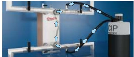
Flush the BPHE with water, starting from the lower connection until it is neutral (pH 7).
