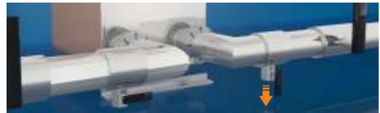
Stop the CIP machine. Drain the BPHE and CIP machine of cleaning agent.
