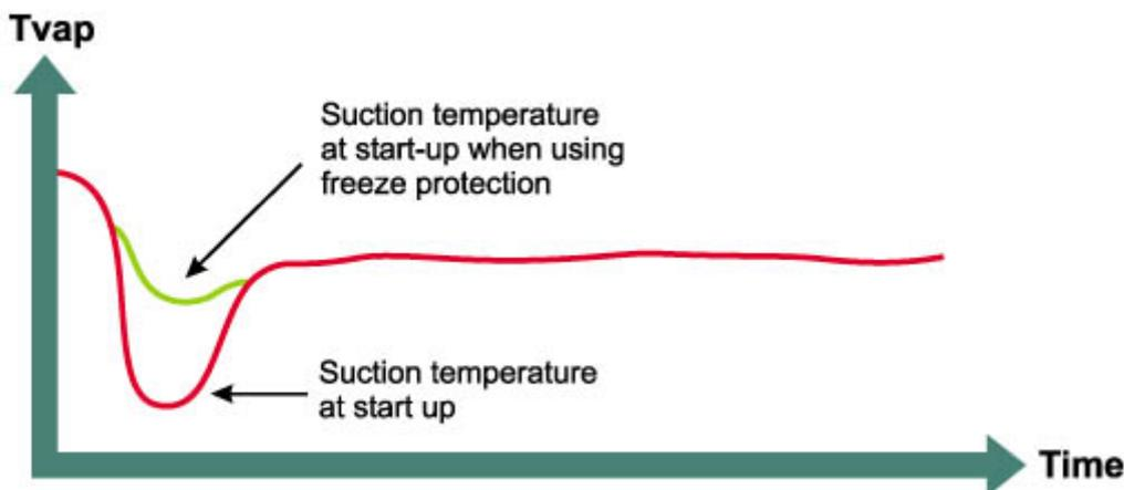
Figure 1. Suction temperature at start up, with and without protection against freezing
