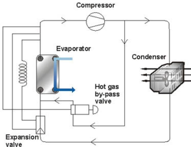
Figure 3. Refrigerant system with freezing control using a hot gas bypass valve on the refrigerant side.
