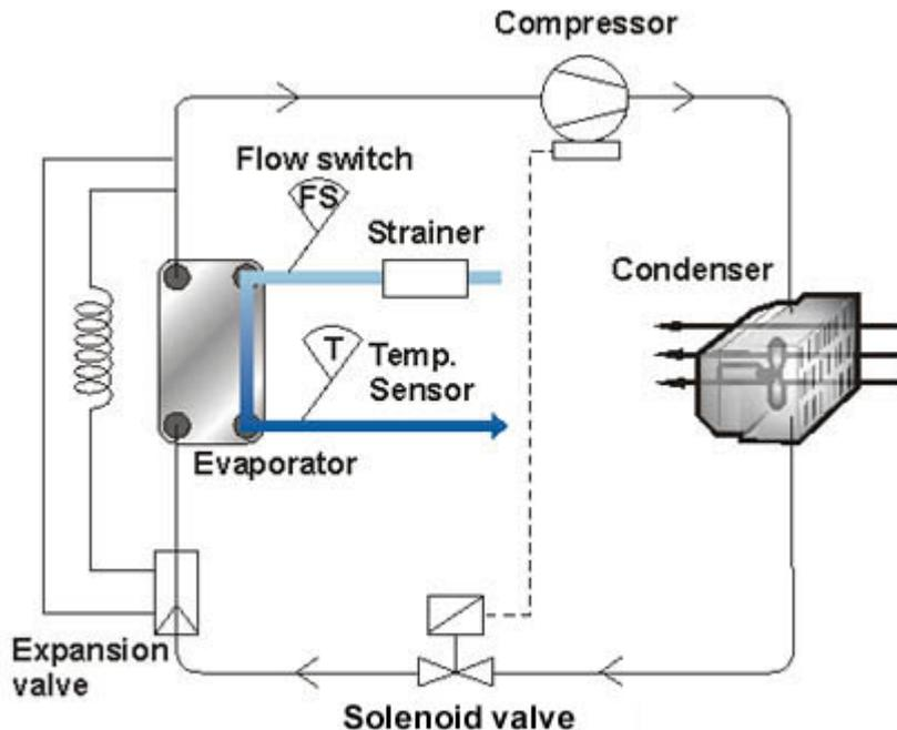
Figure 2. Refrigerant system that can be prevented from freezing by controlling the water side.
