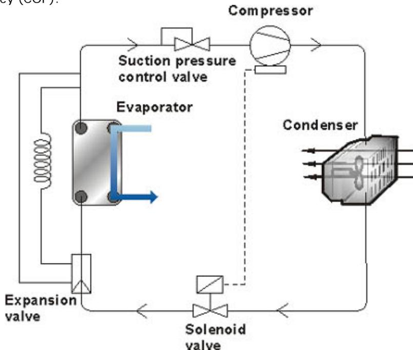
Figure 4. Refrigerant system with freezing control using a suction pressure control valve on the refrigerant side.
