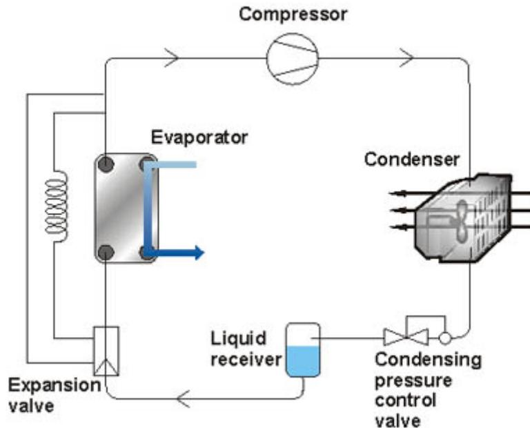
Figure 5. Refrigerant system with freezing control using a condensing compressor control valve on the refrigerant side.
