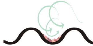
Figure 2. An illustration of how the turbulent flow and shear stresses help keep the BPHE clean.
